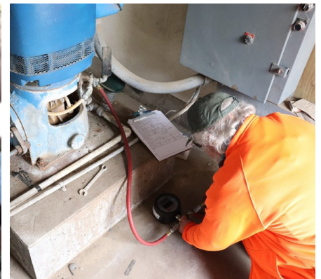
Left: Conservation district staff use an E-tape to measure the water level of a domestic well. Right: Staff measuring the water level of an irrigation well.
