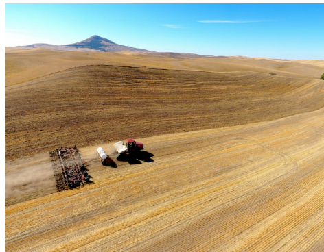
A producer uses GPS guided precision agriculture systems to fertilize his winter wheat. He estimates 6.5 percent reduction in overage.
