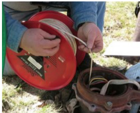
Left: Conservation district staff use an E-tape to measure the water level of a domestic well. Right: Staff measuring the water level of an irrigation well.
