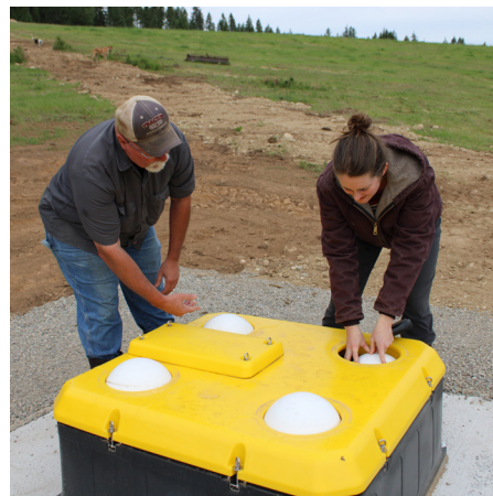
Landowner, Kevin Bush, and POCD Manager, Alex Case-Cohen, observing the float ball action of the new frost-free water tank. (photo by Mary Malone)
