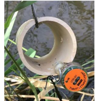
Deploying a temperature logger at Foster Creek.
